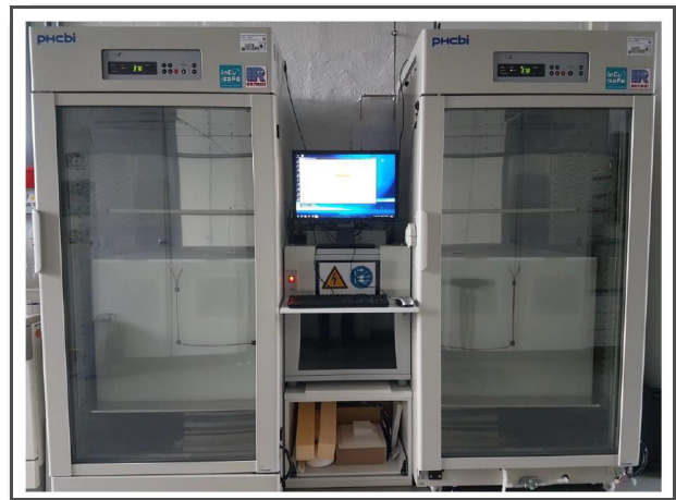
Experimental setup for 5G electromagnetic field exposure of human cells. The incubators ensure constant temperatures.
